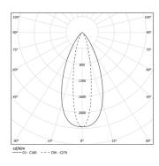
Angle du faisceau Elliptical 22×47° Application
