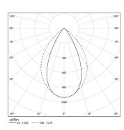
Beam angle Wide flood 76° Application Weight
