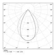
Beam angle Wide flood 76° Application Weight
