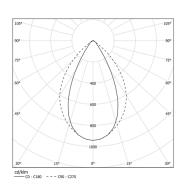
Beam angle Wide flood 76° Application Weight
