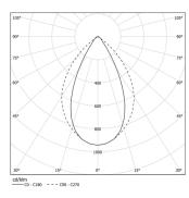
Beam angle Wide flood 76° Application Weight
