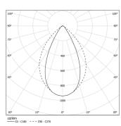
Beam angle Wide flood 76° Application Weight
