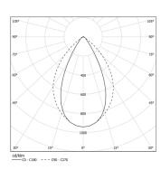
Beam angle Wide flood 76° Application Weight
