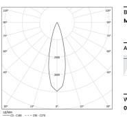
Beam angle Medium 26° Application Weight 0.08Kg
