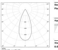
Beam angle Flood 42° Application Weight 0.08Kg cd/klm C0 - C180 --- C90 - C270
