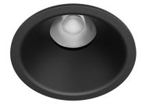
Design: O/M Ceiling-recessed luminaire made of aluminium diecast. Recessing system with spring clips. Recessing accessory for flush version supplied
