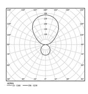
Beam angle Diffuse Direct/ Indirect
