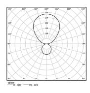
Beam angle Diffuse Direct/ Indirect
