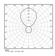
Beam angle Diffuse Direct/ Indirect
