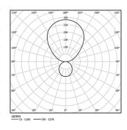
Beam angle Diffuse Direct/ Indirect
