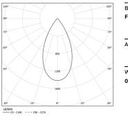
Beam angle Flood 50° Application Weight 0,6Kg
