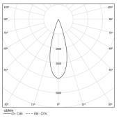
Beam angle Medium 30° Application Weight 0,6Kg
