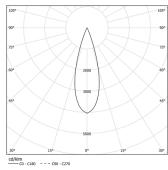
Beam angle Medium 31° Application Weight 1,9Kg
