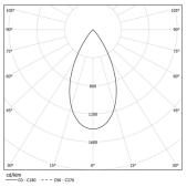
Beam angle Flood 52° Application Weight 1,3Kg
