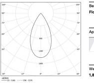
Beam angle Flood 52° Application Weight 1,8Kg
