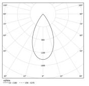
Beam angle Flood 52° Application Weight 1,8Kg
