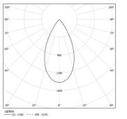
Beam angle Flood 52° Application Weight 1,8Kg
