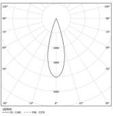
Beam angle Medium 31° Application Weight 1,8Kg
