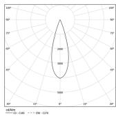
Beam angle Medium 31° Application Weight 1,8Kg
