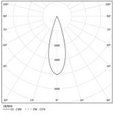
Beam angle Medium 31° Application Weight 1,8Kg
