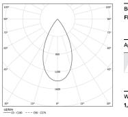
Beam angle Flood 52° Application Weight 1,8Kg
