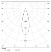
Beam angle Medium 31° Application Weight 1,8Kg
