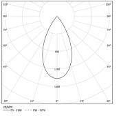
Beam angle Flood 52° Application Weight 1,8Kg
