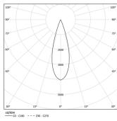
Beam angle Medium 31° Application Weight 1,8Kg
