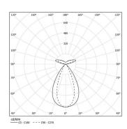
Beam angle Flood 64° / batwing
