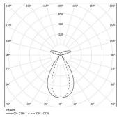
Beam angle Flood 64° / batwing Application
