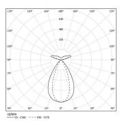
Beam angle Flood 64° / batwing
