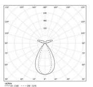
Beam angle Flood 64° / batwing Application
