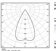
Beam angle Flood 56° Application Weight 0,20Kg
