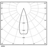
Beam angle Medium 31° Application Weight 0,15Kg
