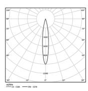
Beam angle Spot 15° Application Weight 0,64Kg
