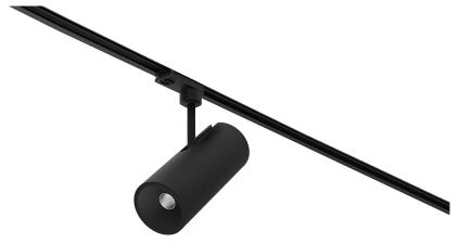
Design: O/M + Bartenbach GmbH Track-mounted spotlight with die-cast aluminium body with electrostatic 100% polyester paint finish. Spot-lens with individual complex surface rips to provide a focal light and an extremely narrow beam. Orientable by 90° horizontal rotation and 330° vertical rotation.
