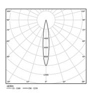
Beam angle Spot 15° Application Weight 0,64Kg
