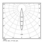
Beam angle Spot 15° Application Weight 0,64Kg
