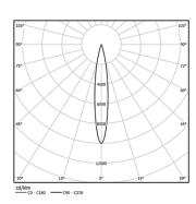
Beam angle Spot 15° Application Weight 0,64Kg
