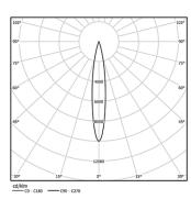
Beam angle Spot 15° Application Weight 0,64Kg
