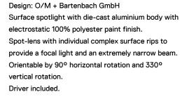
LED CRI>80 / >50.000h, L80/B10 2-step MacAdam / Power supply included. IP20 | 230Vac | 50/60Hz
