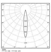
Beam angle Spot 15° Application Weight 0,64Kg
