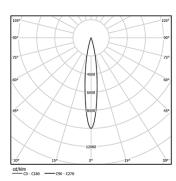
Beam angle Spot 15° Application Weight 0,64Kg
