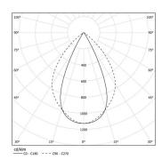
Beam angle Wide flood 80° Application Weight
