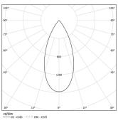
Beam angle Flood 46° Application Weight
