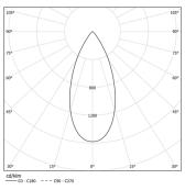
Beam angle Flood 46° Application Weight
