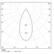
Beam angle Flood 46° Application Weight
