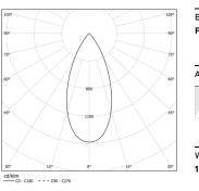
Beam angle Flood 46° Application Weight
