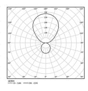
Beam angle Diffuse Direct/ Indirect
