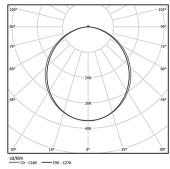
Beam angle Diffuse Application Weight 13Kg
