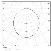
Beam angle Diffuse Application Weight 5Kg
