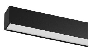
Design: Eduardo Souto de Moura Surface or pendant luminaire with housing made of aluminium profile with 25micron maximum corrosion resistance anodization with matt finish or with textured electrostatic 100% polyester paint. Frosted polycarbonate diffuser with user friendly clipping system and double fitting system: flushed or recessed.
