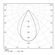
Beam angle Wide flood 80° Application Weight
