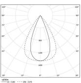
Beam angle Flood 65° Application Weight
